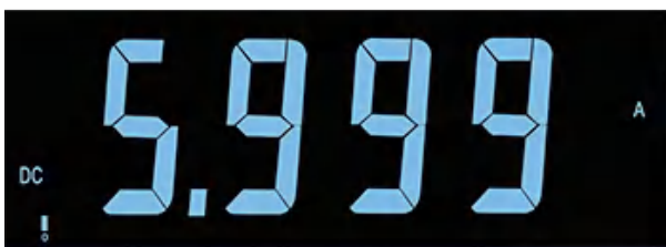
● Reading resolution 3%, maximum reading 5999
