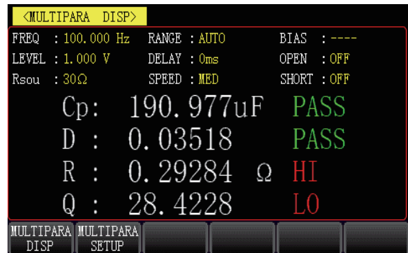
● Multi-parameter display, multiple parameter measurement results can be seen at the same time
