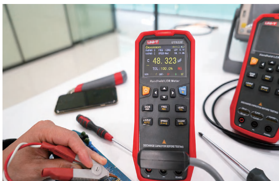
● Tolerance mode used for component sorting
