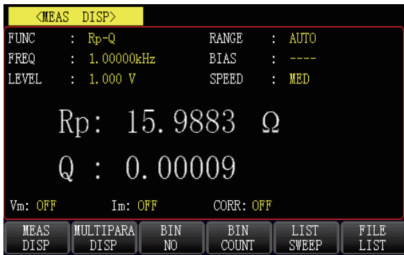
● 4.3-inch full-color LCD display, clear measurement parameters and data
